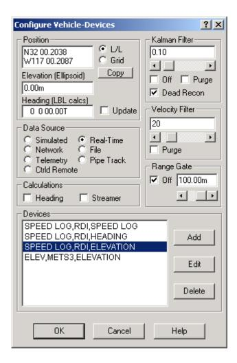
In order to utilize the SPEED LOG data in the determination of the vehicle position, the Kalman Filter must be on, i.e. not checked *Off.*
