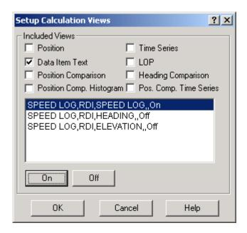
Select the *Data Item Text* checkbox, highlight the SPEED LOG item and then click the *On* button. Exit with *OK*. The speed log data can then be monitored in this Calculation Window, as shown below.
